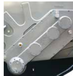
Dual transmission with side gearbox increase power delivery to the rotor
