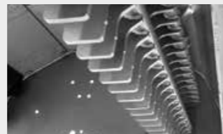
Independent Grid for control of finer product; increased distance between the grid and the rear door allows a better material flow
