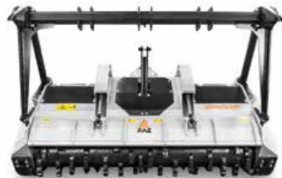
UMM/S Forestry mulchers for PTO tractors with fixed tooth rotor.
