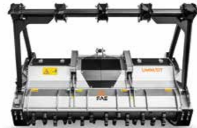
UMM Forestry mulcher for PTO tractors with fixed tooth rotor.
