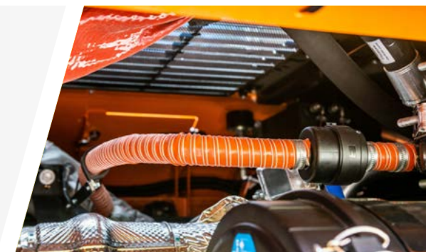
Heavy-duty filtration system (ejector)
