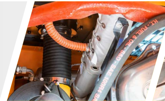
Heavy-duty filtration system (ejector)
