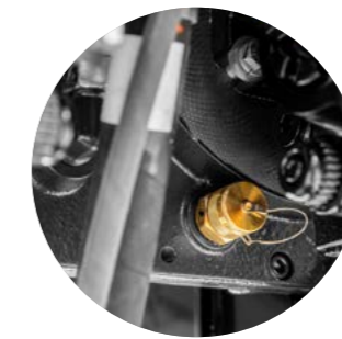
Couplings make it possible to quickly drain fluids without leaks (5)
