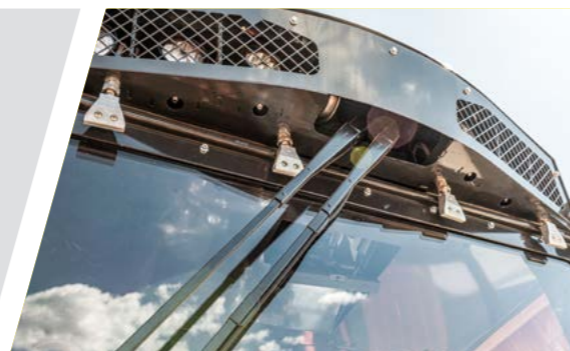
Air window cleaning system
