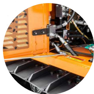
The large rear doors have safety catches (2)
