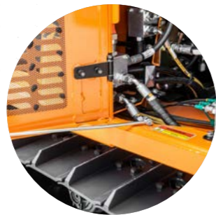
The large rear doors have safety catches (2)
