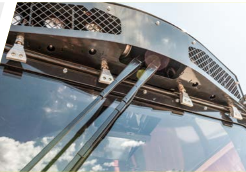
Air window cleaning system
