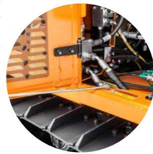
The large rear doors have safety catches (2)
