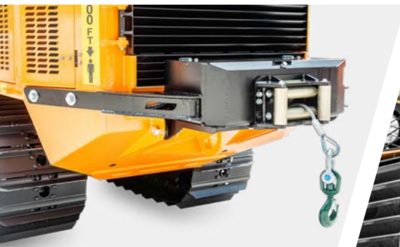
Rear winch with 6-tpulling force
