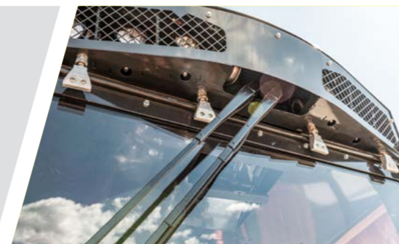
Air window cleaning system
