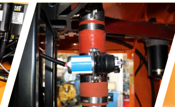
Air shut-off system
