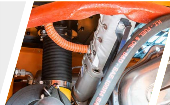
Heavy-duty filtration system (ejector)
