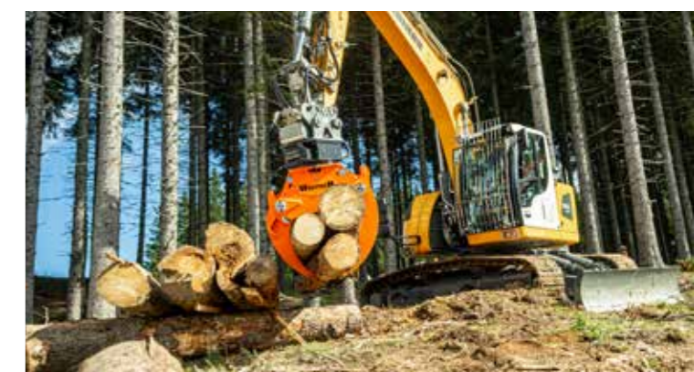
Gripper opening stroke 1270mm.
