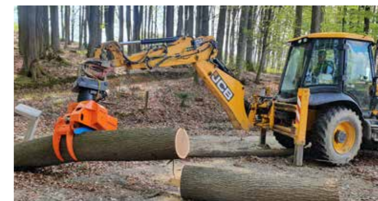
Sturdy and low-wear woodgripper with saw unit.
