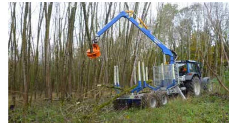
CB150 crane suitable for forest crane attachment.
