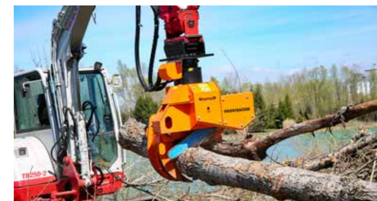
Can be mounted to cranes, timer trailers or excavators.
