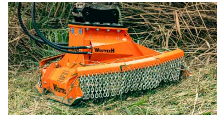
Easily replaced knives, replaceable attrition skids.
