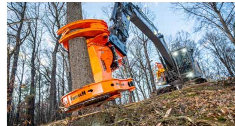
C650 with cutting diameter up to 70 cm.
